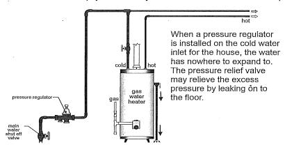
This doesn't happen every time that a pressure reducing valve or check valve is installed, but there may be other problems that show up in the house, such as the toilet fill valves randomly refilling toilets, or faucets chronically dripping.
