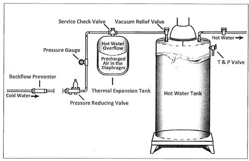
shown close to the water heater. The installation may or may not have a pressure reducing valve. The installation of a pressure reducing valve will not prevent thermal expansion.
